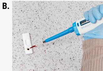
B. Hold the pipette vertically and dispense the specimen into the sample well.
